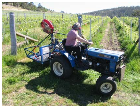
Figure 8. Spray application in 2004. (a) Small plot air-blast sprayer in action on 18 October 2004. The sprayer was built and operated by Dr Gordon Brown, Scientific Horticulture Pty Ltd, Tasmania.
