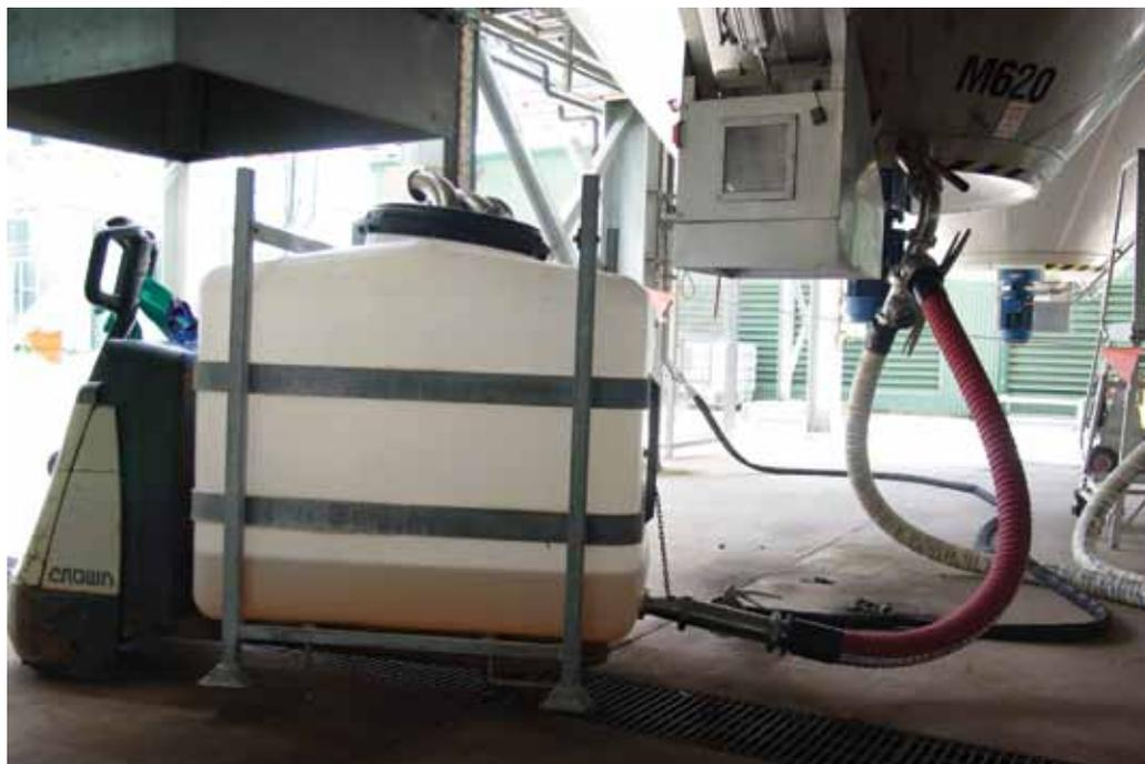
Mobile tank cleaning unit in use at Oxford Landing.
