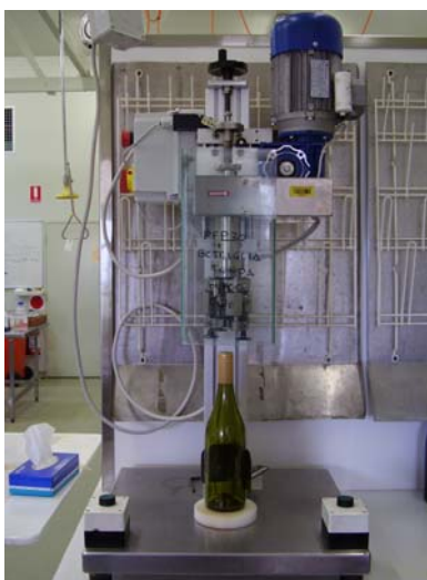
Figure 9. Screw capper used in sealing wine in bottles
