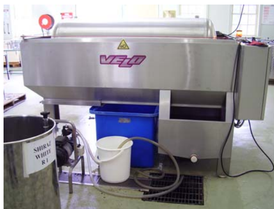
Figure 5. The Velo 600 Litre tank press used for pressing wine
