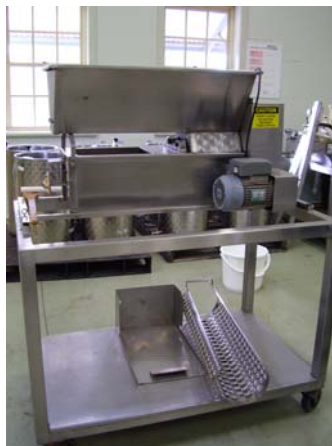
Figure 7. Crusher/destemmer used for processing grapes
