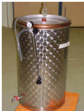
Figure 4. Variable capacity stainless tanks with lids showing seals
