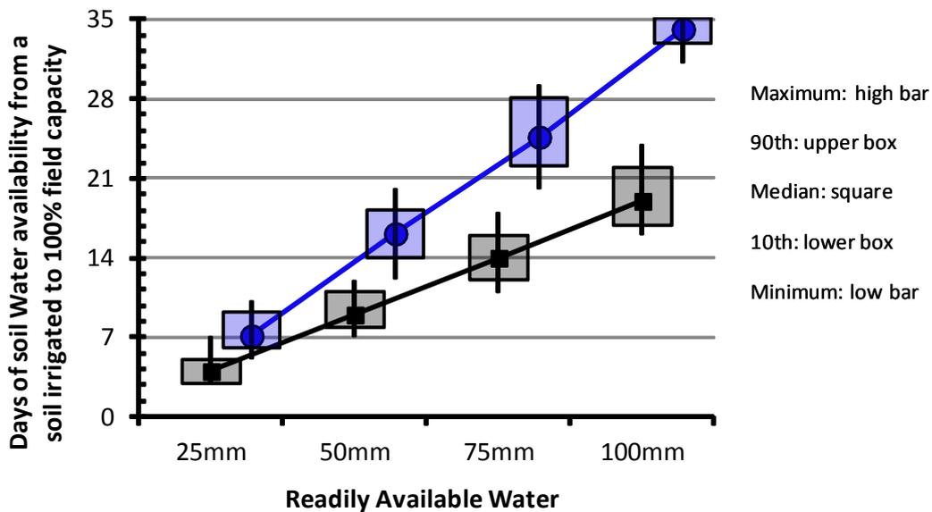
**Figure 6.** Days that a fully irrigated soil on 15 February with RAW from 25 to 100mm can supply water requirements to a vine at Nuriootpa. Black lines and boxes when crop coefficient is 1.0; Blue
