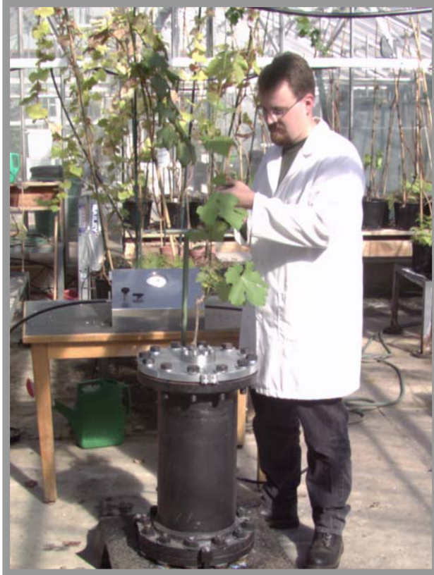
Figure 1. Grapevine inserted in a root pressure chamber for sap collection.
