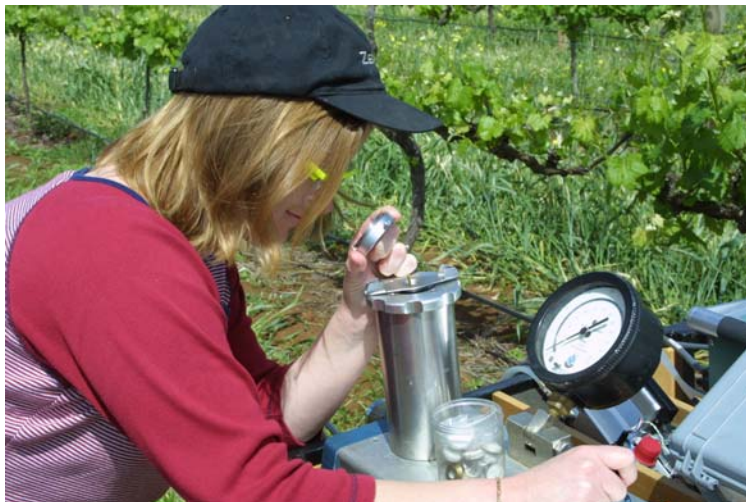
Figure 2. Scholander-type pressure chamber used for routine measurement of leaf water potential and collection of petiole sap.
