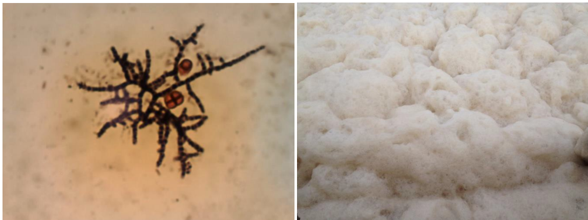
Figure 6.1.5 GALO with typical right angle branching and thick viscous foam.
