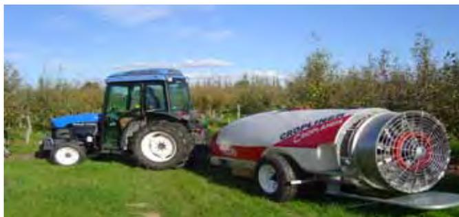
Angle row airblast sprayer with large rear axial fan.
