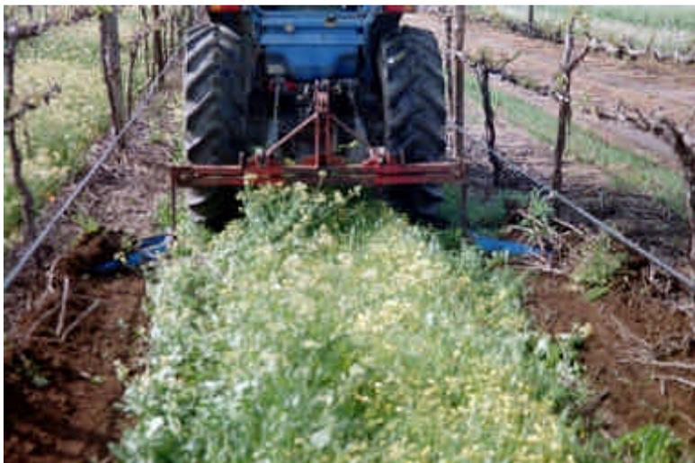
**Plate 4:** The Bezzerides under-vine weeder being evaluated in a Langhorne Creek vineyard.
