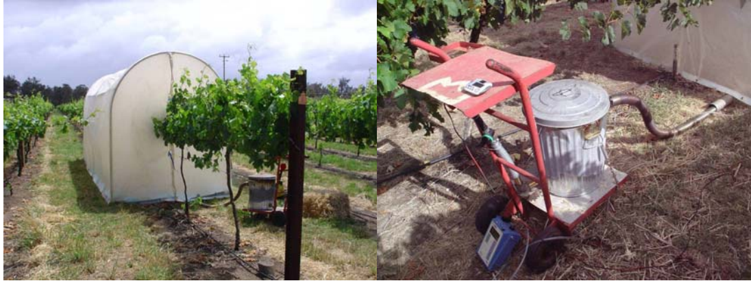
Figure 2. Field smoke application apparatus showing smoke tent with vines enclosed (left) and smoke generator (right).
