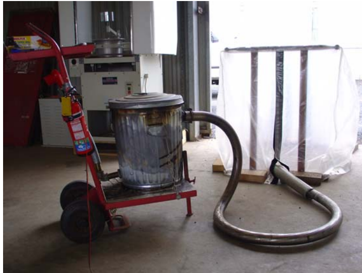
Figure 4. Small scale model for the application of smoke to grape berries. Apparatus utilises smoke generating equipment and a small scale tent.
