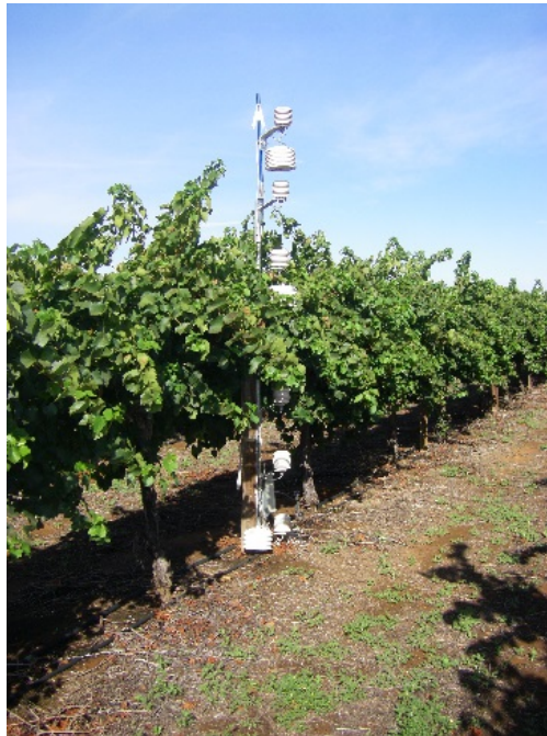
Figure 2. Temperature and relative humidity recording mast located in the Ricca Terra trial site near Barmera, SA.
