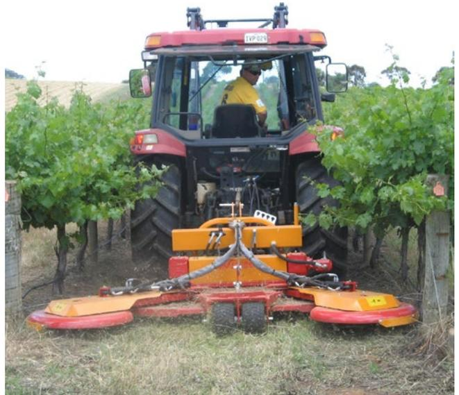
**Figure 3:** Mowing the mid-row and undervine simultaneously is an efficient non-chemical weed management strategy.
