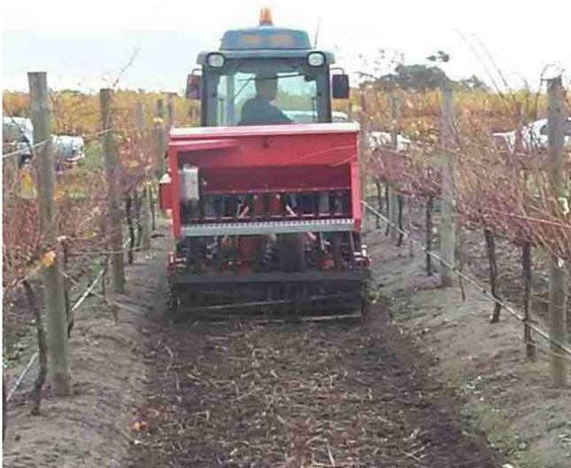
**Figure 1:** A power harrow fitted with a seed box and compaction roller is an alternative seeding system to the traditional tyne- or disc-based drill.
