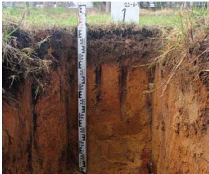
8. Leachfields are biological systems that rely on microbial treatment within the soil column and the bulk of the microbes are at or close to the surface. Leachfields should therefore be as shallow as legally possible (150 mm minimum below ground level AS/NZS 1547) as wastewater discharged below the upper aerobic soil layer tends to have little or no treatment which can result in discharge of high-strength winery wastewater to groundwater (Crites & Tchobanoglous, 1998).
