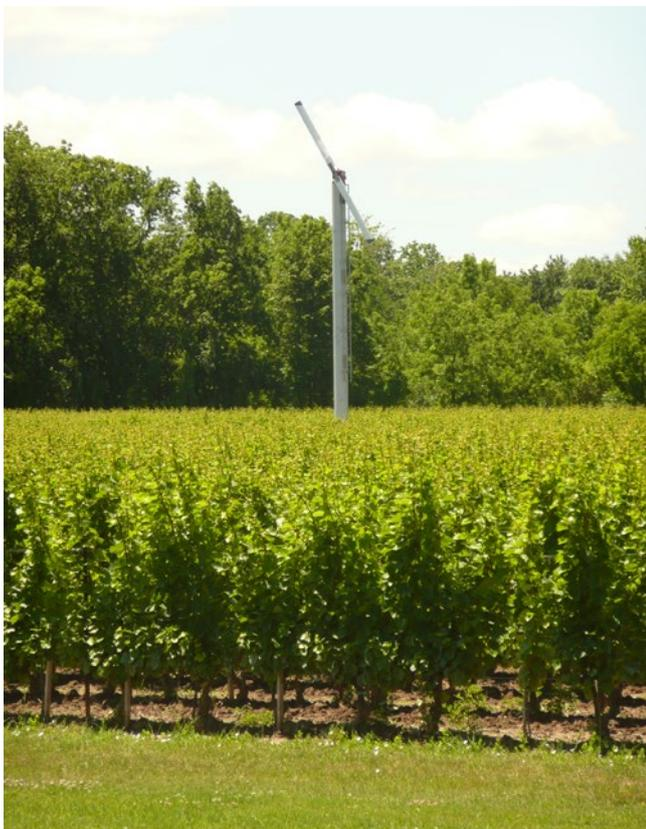
**Figure 3:** A frost fan in the Niagara region of the US. (Photo courtesy of Hans Loader).
