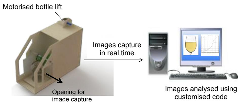
**Figure 4:** Robotic pourer kit and associated image analysis layout to assess quality of sparkling wine.
