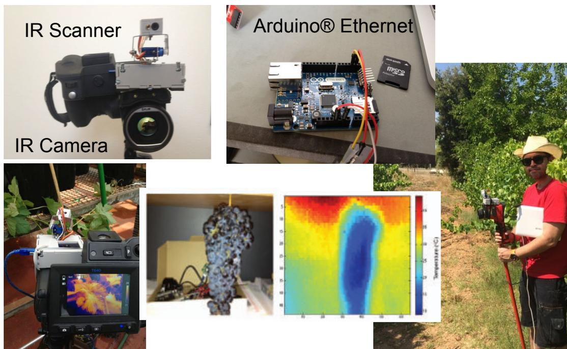
**Figure 3:** Low cost Infrared scanner kit compared to a high resolution infrared camera.
