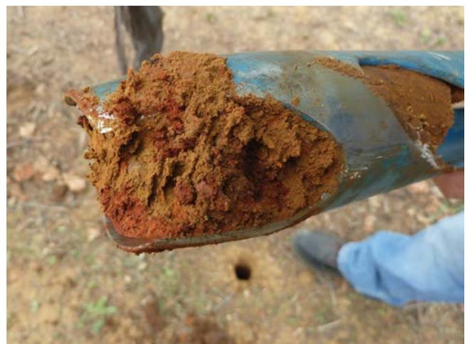
Figure 1: Using an auger to collect soil samples in the field.
