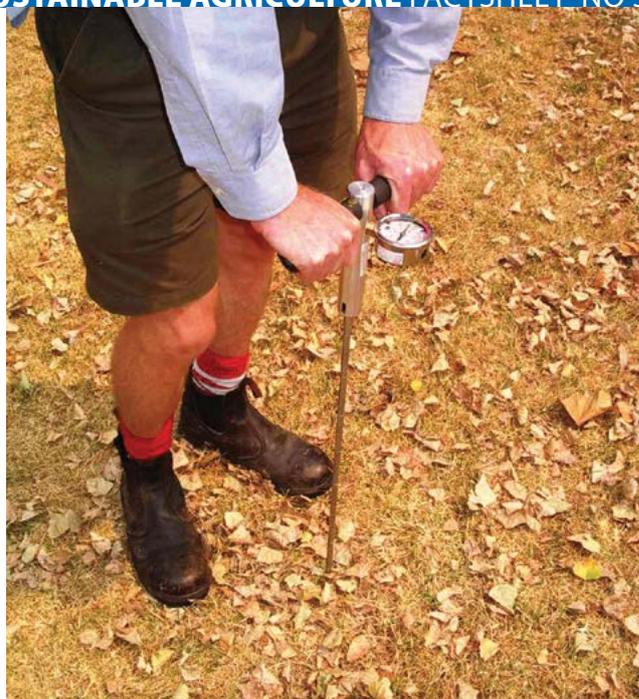
Figure 7: Assessing soil strength in the field using a penetrometer. (Photo: R.E. White)
