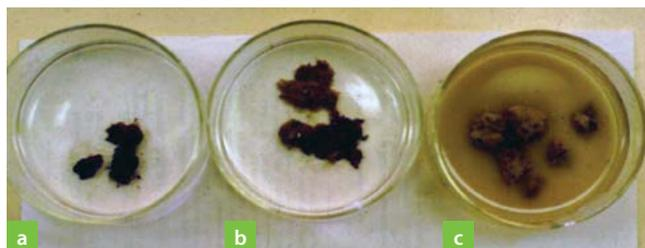
Figure 6: Assessing aggregate stability in the laboratory (a) aggregates remain stable (b) aggregates swell and slake (c) aggregates swell, slake and disperse. (Photo: DEPI, Victoria)
